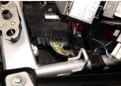
Splice the SpeedoHealer Red wire to the Orange wire of the rear brakelight switch connector.
