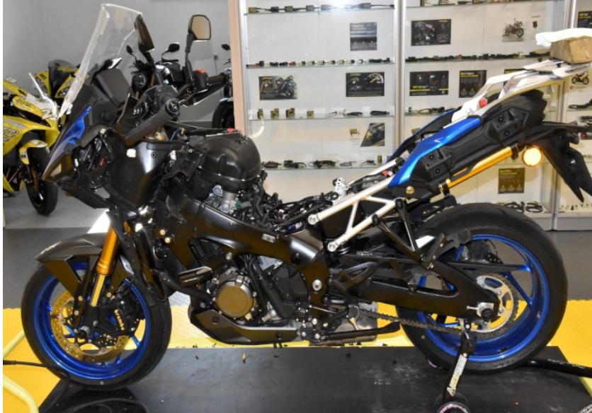
Locate the ABS module under the fuel tank and locate the ECU on the airbox.
