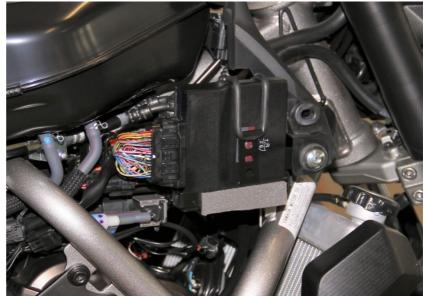
Cut the White/Yellow (speed signal) wire at the ECU connector.
