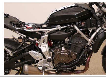
Locate the ECU connector below the fuel tank.
