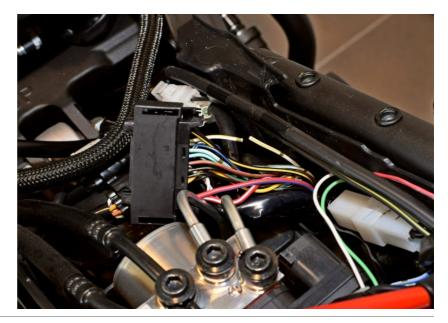
Splice the SpeedoHealer White wire to the White/Yellow wire end, which goes to the ABS ECU connector.
