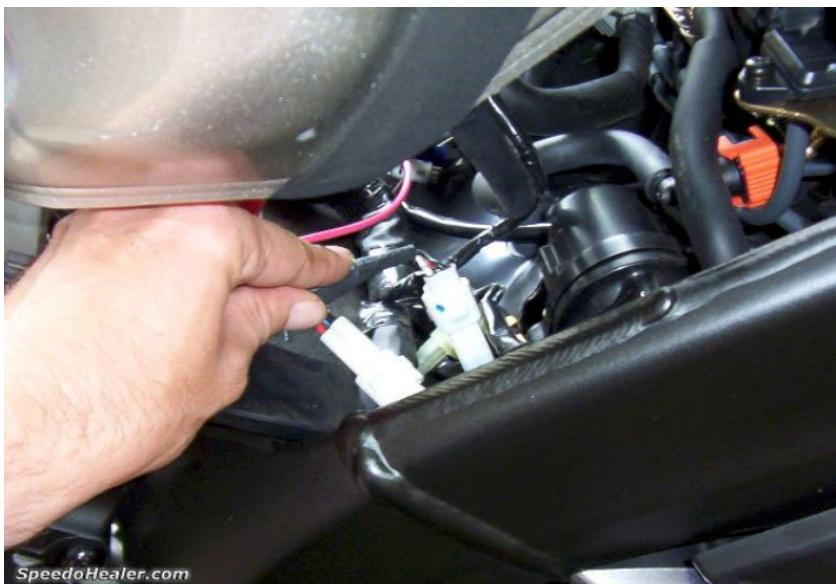
Locate the vehicle speed sensor connectors.
