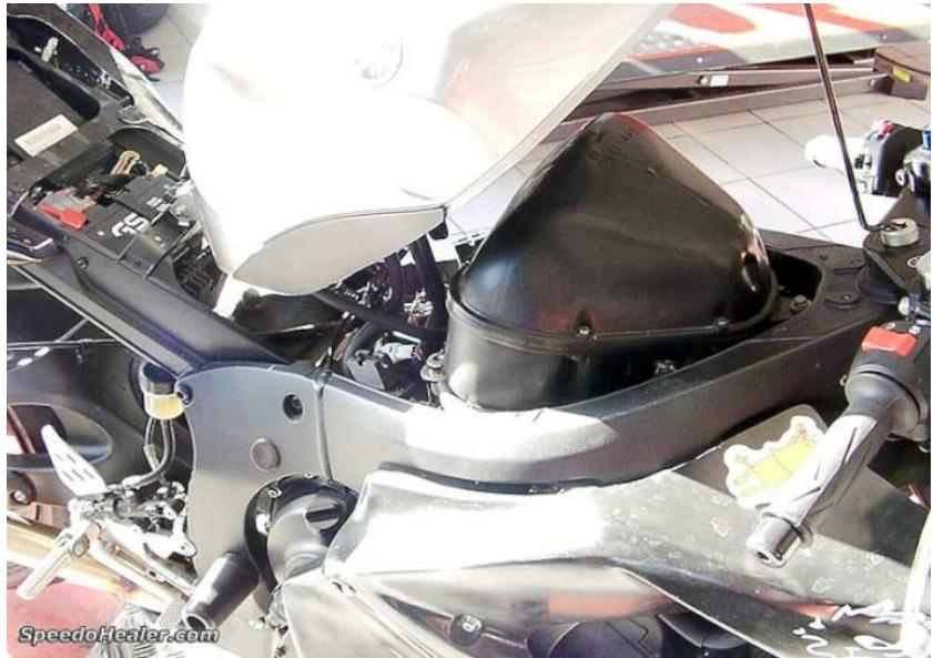
Locate the vehicle speed sensor connectors.
