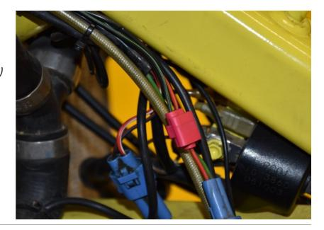
Connect the SLP Black wire to the ignition coil Brown wire (ground terminal).
