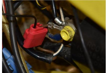
Connect the SLP Red wire to the battery positive terminal via an on/off switch.
