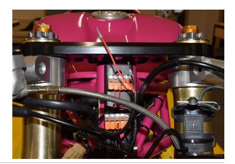
Typical position of the Shift Light Pro, battery and the on/off switch.
