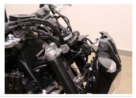
Remove the fairing around the fuel tank and the plastic cover on the right side.
