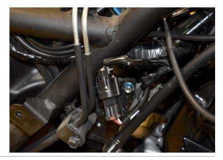
Find the Sub-throttle valve actuator and plug the STVE module into the 4-pole White wiring harness connector.
