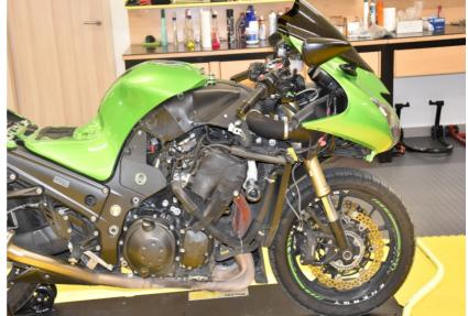
Locate the throttle body assembly under the airbox.
