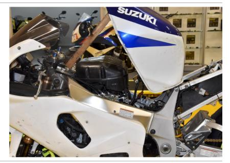
Locate the throttle body assembly under the fuel tank.
