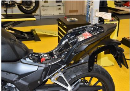
Connect the TB terminals directly to the battery terminals.
