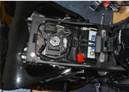
Release and remove the middle two pins from the female connector.
