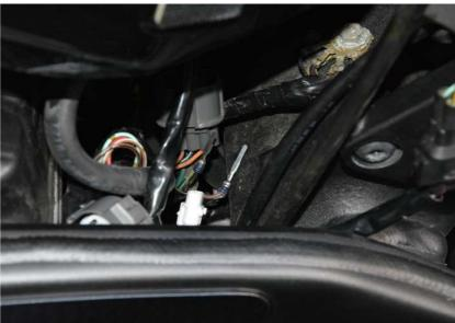
Insert the two male metal contacts into the larger 2-pole plug through the back until they click into place.
