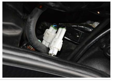
Locate the ECU wiring harness under the main seat, under the rear frame.
