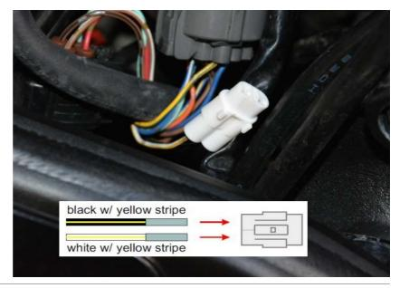
Release and remove the middle two pins from the male connector.
