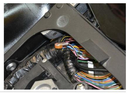
Connect the X-TRE Red wire to the Brown wire of the rear brake light switch connector.
