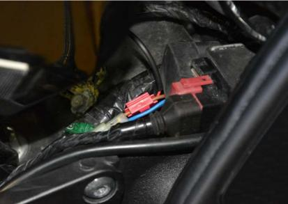
Typical position for the X-TRE Power Box module.
