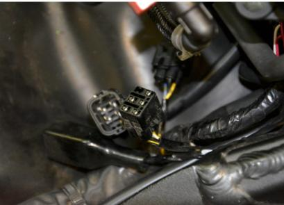
Release and remove two terminals from the smaller, 6-pole connector.
