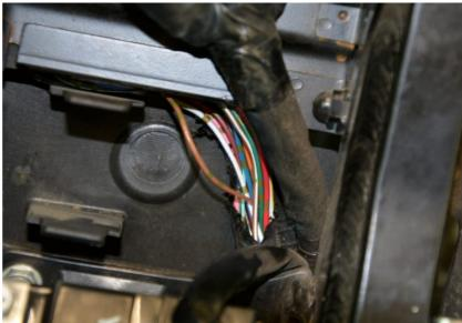
Connect the X-TRE Black/Green wire to the Brown/Red wire end, which goes to the ECU connector.
