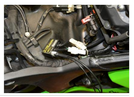
Locate the ECU wiring harness connector under the main seat, under the starter relay.
