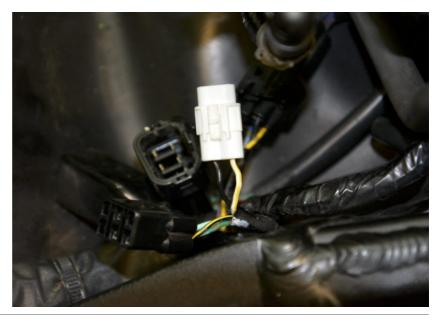
Release and remove two terminals from the larger, 6-pole connector.
