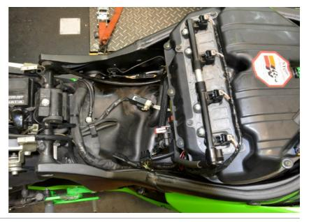
Unplug the Gear Position Sensor connector.
