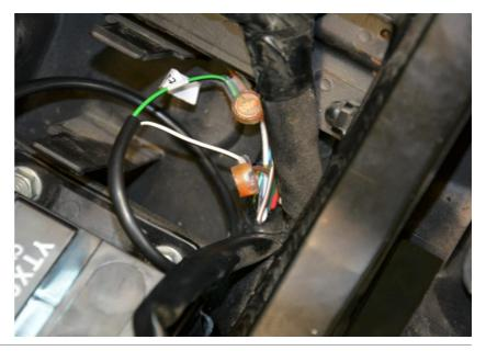
Connect the X-TRE Red wire to the Red/Blue wire of the rear brake light switch connector.
