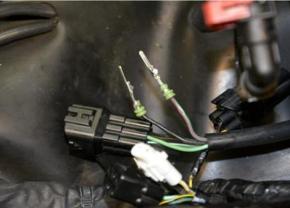
Insert the Black and Green/Red wires into the larger white, 2-pole connector.
