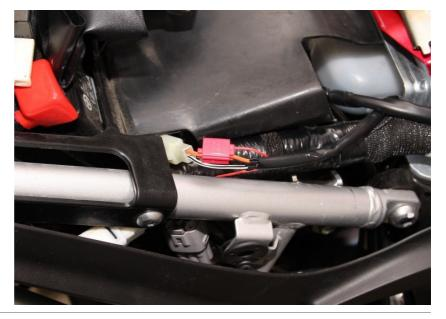
Mount the X-TRE box to the inner side of the side fairing by the supplied Velcro strips, and secure the box and cables with cable ties.
