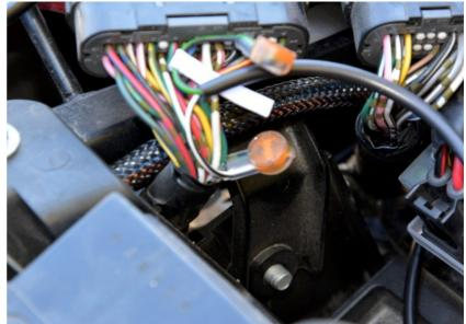
Connect the X-TRE Red wire to the Orange wire of the rear brake light switch connector.
