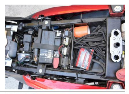
Plug the X-TRE connectors in-line with the gear position sensor connectors.
