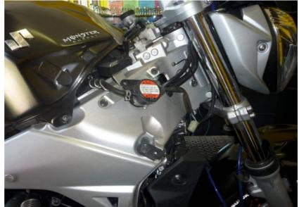
Lift up or remove the fuel tank.
