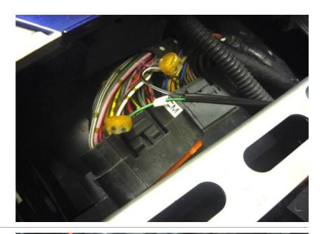
Connect the X-TRE Red wire to the Orange/Green wire of the rear brake light switch connector.
