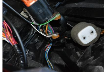
Connect the X-TRE Red wire to the Orange/Green wire of the rear brake light switch connector.
