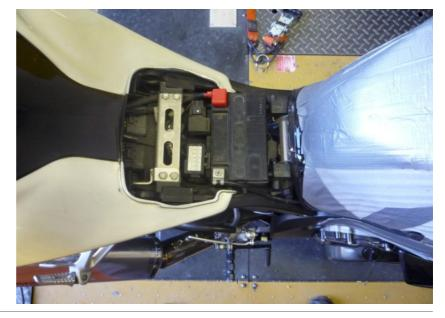
Lift up or remove the fuel tank.
