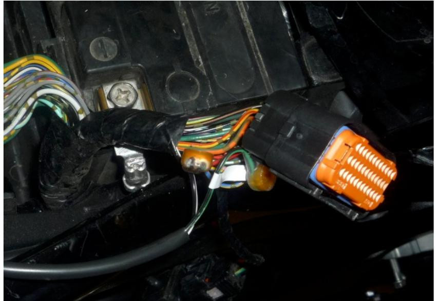
Connect the X-TRE Red wire to the Orange/Green wire of the rear brake light switch connector.
