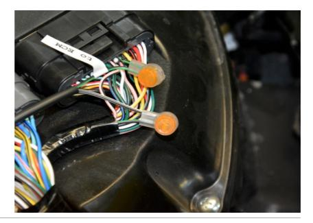
Connect X-TRE Red wire to Orange wire of rear brake light switch connector.
