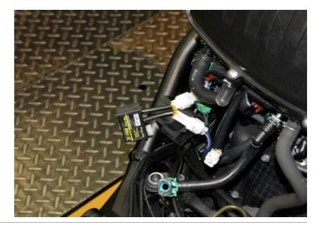
Mount the X-TRE box to the inner side of the frame by the supplied Velcro strips, and secure the box and the cables with the cable ties.
