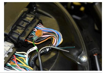
Connect the X-TRE Black/White wire to the Black/Green wire end, which is at the wiring harness side.
