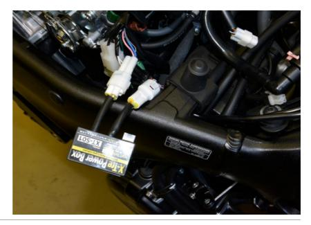
Mount the X-TRE box to the inner side of the frame by the supplied Velcro strips, and secure the box and cables with cable ties.
