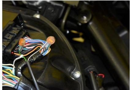
Connect the X-TRE Red wire to the Orange wire of rear brake light switch connector.
