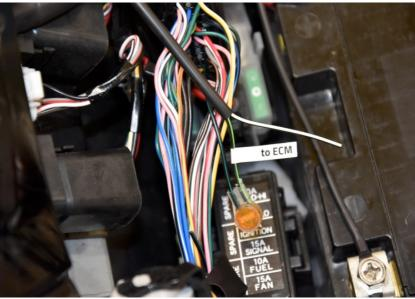
Connect the X-TRE Black/White wire to Black/Green wire end, which is at the wiring harness side.
