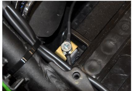
Locate the black ABS module connector under the fuel tank.
