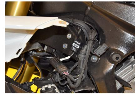
Locate the 2nd Exhaust Servo motor.
