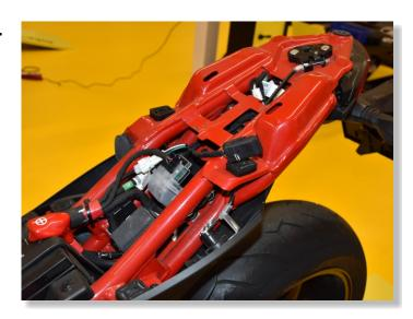
LIFT UP OR REMOVE THE FUEL TANK.
