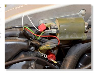
SPLICE THE QSH WHITE WIRE TO THE YELLOW/BLUE OR BLUE/YELLOW WIRE OF THE COIL BY USING THE SUPPLIED RED WIRE TAP CONNECTOR.
