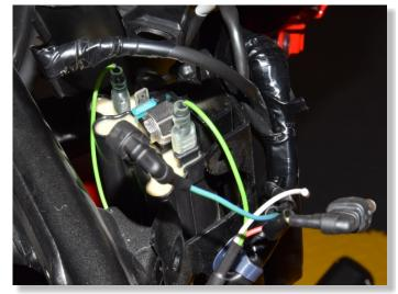
SPLICE THE QSH WHITE WIRE TO THE GREEN/BLUE WIRE OF THE COIL BY USING THE SUPPLIED RED WIRE TAP CONNECTOR.
