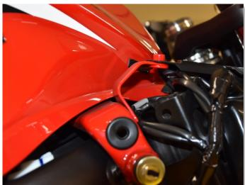
REMOVE THE FUEL TANK AND LOCATE THE IGNITION COIL TERMINALS ON THE RIGHT SIDE.
