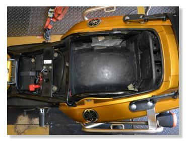
LIFT UP OR REMOVE THE FUEL TANK.
