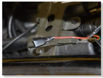
SPLICE THE QSH WHITE WIRE TO THE GRAY WIRE OF THE COIL BY USING THE SUPPLIED RED WIRE TAP CONNECTOR.
