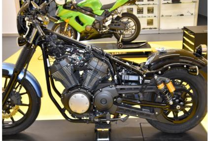
Locate the ignition coil terminals under the fuel tank.
