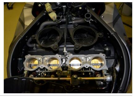
Remove the air intake below the airbox.
