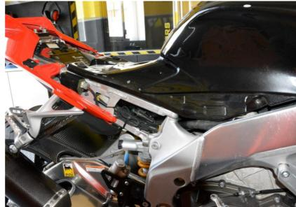
Lift up or remove the fuel tank.
