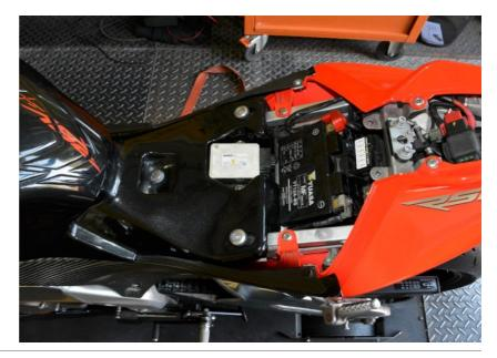
Remove the frame covers below the fuel tank.
