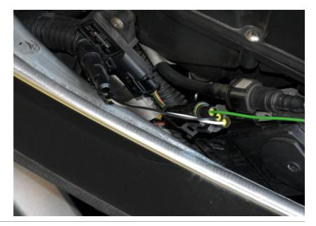
Connect the QSH connectors in-line with the ignition coil connectors on right side.
