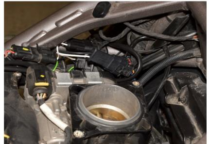
Connect the QSH connectors in-line with the ignition coil connectors on the right side.
