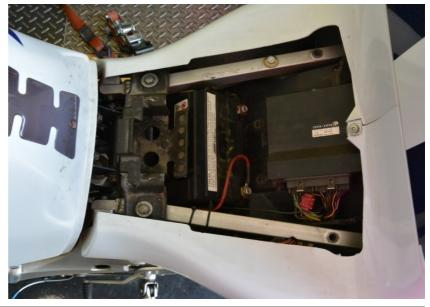
Lift up or remove the fuel tank.
