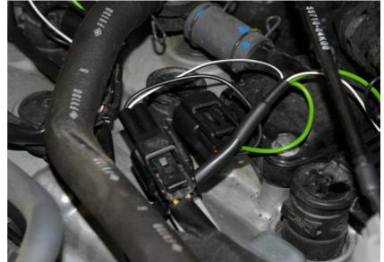
Mount the QSX module to the inner side of the frame by the supplied Velcro strips, and secure the cables with cable ties.
